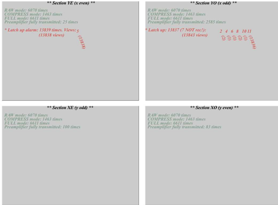
Figure 3: Calorimeter_Detector_Report_3/3. This is the report sheet of the quick-look. Each section has recorded 6070 events in RAW mode, 1463 events in COMPRESS mode and 6611 events in FULL mode. The section YO was the one which transmitted the higher number of times the preamplifier in raw mode (2585) which is about the 30% of the FULL and COMPRESS mode acquisition. In this file there were some latch-up alarms in sections YE and YO. Notice that in the case of section YE the DSP recorded a latch-up alarm 13839 times while CaloQLOOK only 13838 times, one time less since there are some capacitors which take time to discharge and during the first latch-up event that section recorded some data even if the plane was not powered on. The opposite can be noticed in section YO, where the latch up was recorded 13837 times by the DSP but 13843 times by CaloQLOOK. As discussed in section 2.1 the exceeding latch-up alarm are not real latch-up but an effect of the warming up of that section.
